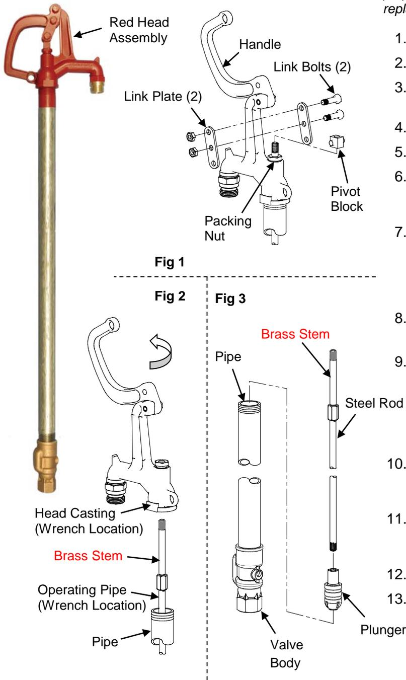
1. Shut off water supply to hydrant.
