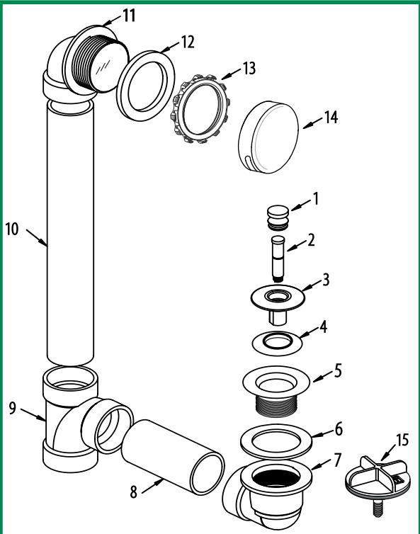
**Step 1:** Cut the 1½" Schedule 40 pipes (**Item 8 and Item 10**) to the desired lengths to fit the tub.
